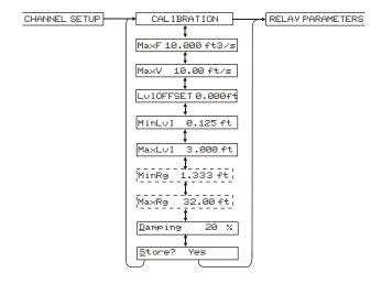
From CAL IBRATION press ♣ to MaxF. Enter the maximum expected flow in your application. If the maximum expected flow is unknown, enter an estimated value.
