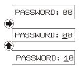
Factory default Password is ØØ. A new password can be stored by going → to SPECIAL FUNCTION and → to New Password.
