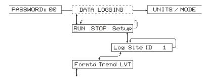
From RUN STOP SETUP press  $\Rightarrow$  to SETUP and then  $\P$  to Log Site ID  $\varnothing$ . Press  $\Rightarrow$  to position the cursor under the numeral and  $\P$  or  $\P$  to change the numerals. The "Site ID" number is retained with data logging sessions to identify logs stored from different locations.
