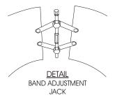
Use optional VSJ stainless steel Pipe Mounting Bands for easy Sensor installation in round pipes.
