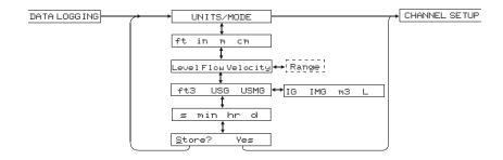
Press → to UNITS/MODE, then → . Press → to move the cursor under the required measurement units:
